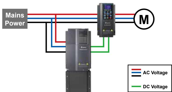
Provides the crane and hoist system four-quadrant operation and energy saving performance with the power regeneration function.
