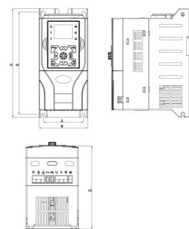
Figure 2-3 Dimensions of Inverter 0.75KW~30KW
