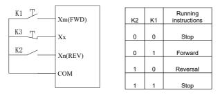
Figure F7-5 Schematic diagram of three-wire control mode 2
