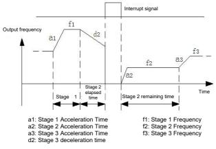
Fig. F9-4 PLC starting mode 1
