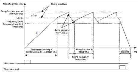
Fig. F9-6 Schematic diagram of Swing frequency
