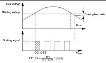
Figure 012-1 Schematic diagram of energy consumption braking
