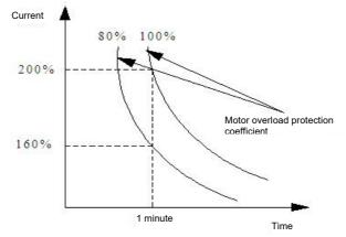
Figure 010-1 Motor overload protection curve
