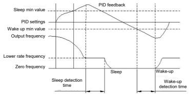
Figure F8-5 Schematic diagram of the first sleep mode
