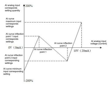
Fig. F6-2 Schematic diagram of multi-point curve
