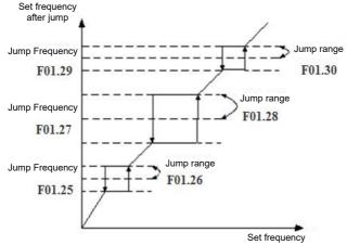
Figure 01-6 Diagram of Jump Frequency
