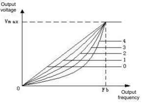
Vmax: Maximum output voltage Fb: Maximum output frequency
