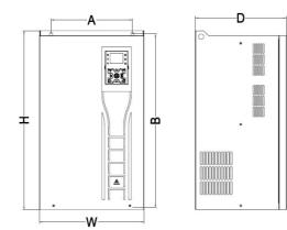
Figure 2-4 Dimensions of Inverter 37KW~220KW
