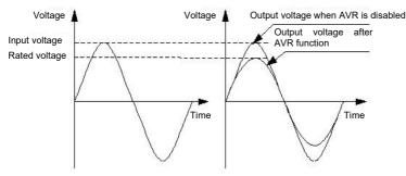
Figure 012-2 Function Diagram of AVR
