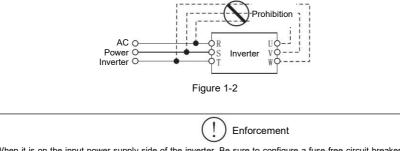
• When it is on the input power supply side of the inverter. Be sure to configure a fuse-free circuit breaker for circuit protection to prevent the accident from expanding due to the failure of the inverter.
