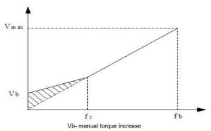
Figure F5-2 Schematic diagram of torque boost
