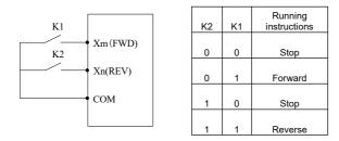
Figure F7-3 Schematic diagram of two-wire control mode 2
