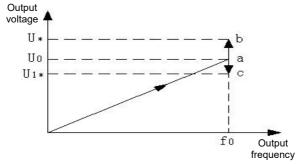
Figure F5-4 Voltage Control Mode 0
