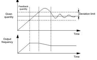
Figure F8-3 Schematic diagram of deviation limit
