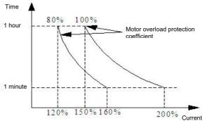
Figure 010-2 Schematic diagram of motor overload protection coefficient setting The motor overload protection coefficient can be determined by the following formula:
