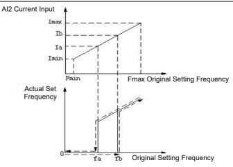
fb :Zero frequency operation threshold fa: fb – zero frequency return difference Figure 56.1 Schematic diagram of zero frequency function
