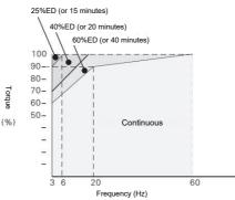
Allowable load characteristics of our standard motor
