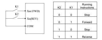
Figure F7-2 Schematic diagram of two-wire control mode 1
