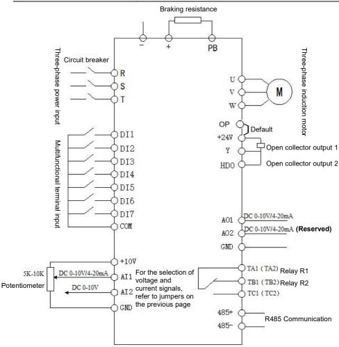
Basic operation wiring diagram
