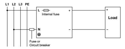
Fig. 5 2 of 3 Phase System Input Operation Connection Diagram
