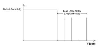
Additionally, if the  $I_0$  is <105-180% but >100% for a prolong period of time (depending on the load), the Over Temperature Protection (OTP) will be activated due to high temperature on critical components. The power supply will then go into "Latch mode" until the PSU cools down and the AC power is recycled.
