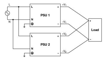
Fig. 3 Parallel Operation Connection Diagram
