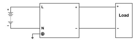
Fig. 4 DC Input Operation Connection Diagram
