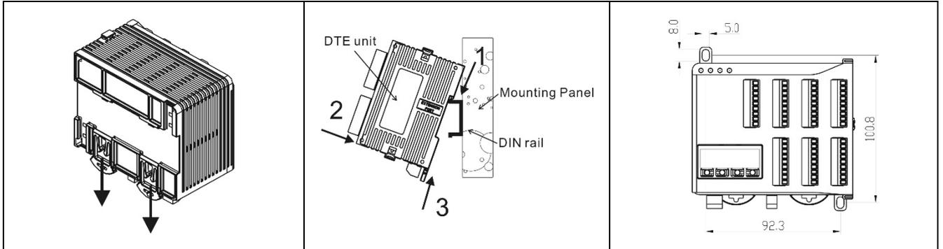
Connect maximum 7 DTC2000 or DTC2001 controllers to DTE by using DIN rail.
