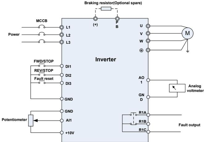
Figure 6 Integrated Wirings
