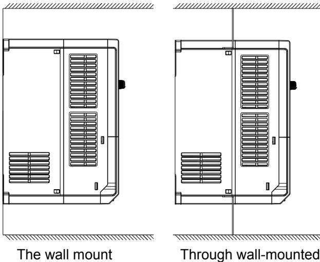
Fig 3-1 Installation methods
