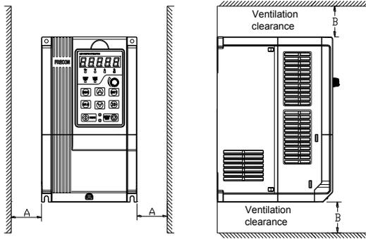
Fig.3-2 Single inverter mounting orientation and space requirements
