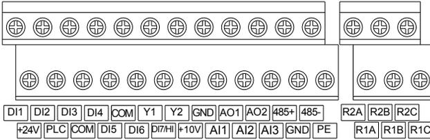
**Figure 3 FR200 series Control Terminal Diagram**
