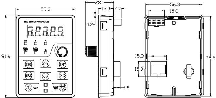
Fig 2-10-a 0.75~2.2KW Keyboard size diagram
