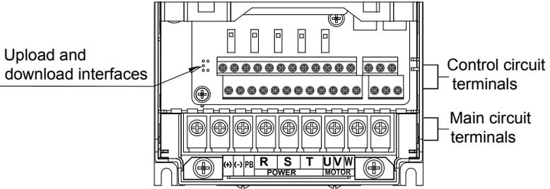
Fig.3-11 0.75~2.2kW Schematic of main circuit terminals
