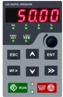
Figure 7 Operation panel diagram
