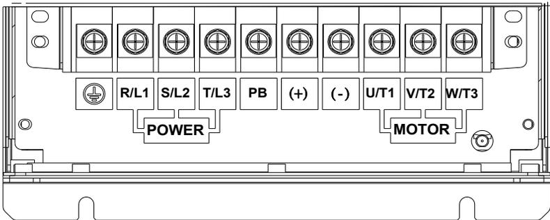
Fig.3-13 18.5~30kW Schematic of main circuit terminals
