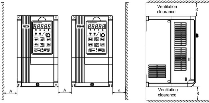
Fig.3-3 multiple inverters installed direction and space requirements
