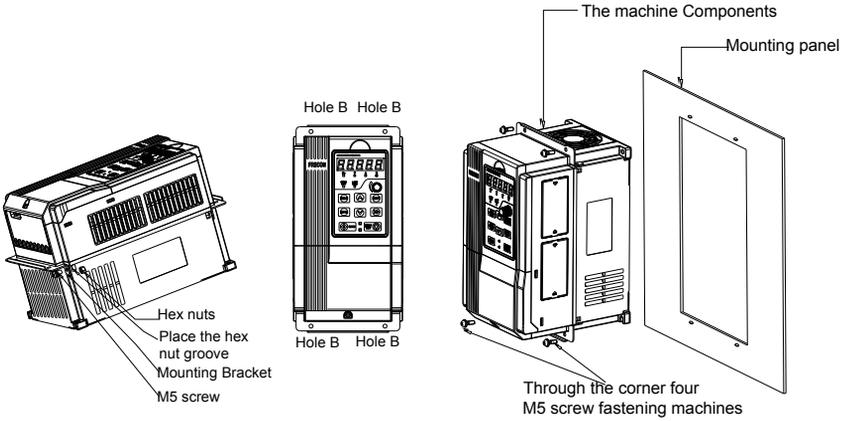
Fig.3-6 (a)0.75~15kW Wall installation
