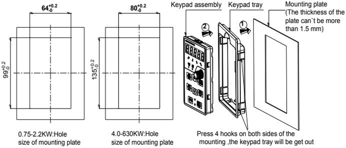
Fig 2-11 0.75~630KW External keyboard installation hole size diagram
