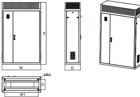
**Fig 2-7 Wall installation diagram**
